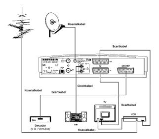
Connection of Sat receiver to TV set and video recorder with coaxial cables.
